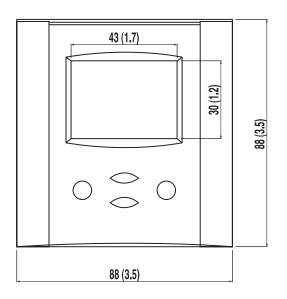
Space required in flush mounting box:  $(H \times W \times D)$
