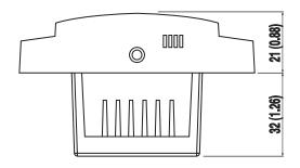
Distance for mounting screws: Horizontal and vertical: 45 to 63mm (1.8 to 2.5 in.)
