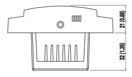
Distance for mounting screws: Horizontal and vertical: 45 to 63mm (1.8 to 2.5 in.)
